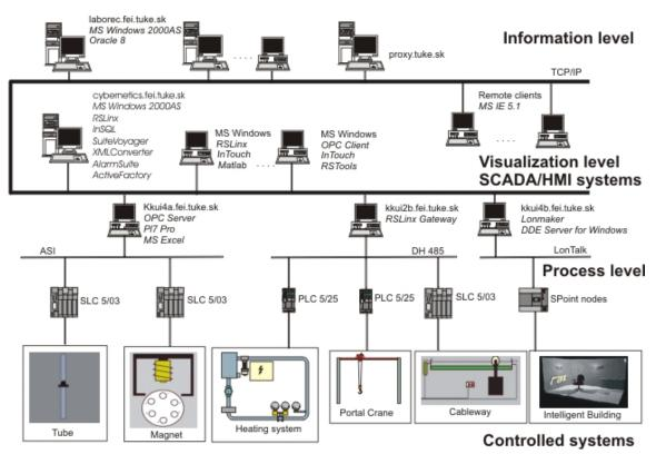
Fig. 1 Physical model ICS of real laboratory models.
