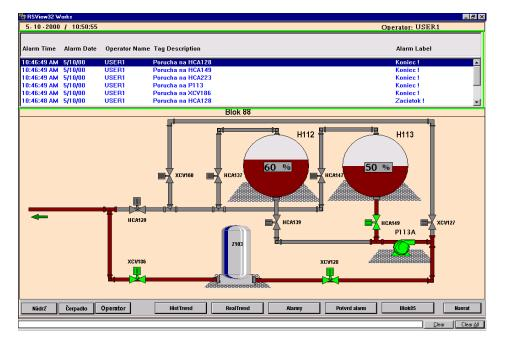
Fig. 4 RSView32 SCADA/HMI, the plant model has been used as a source for real-time process data for a RSSQL configuration and in two web-based monitoring applications
