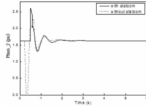
Fig.14: generator 2 active power
