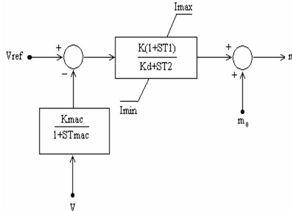
Fig.4: STATCOM voltage control block diagram
