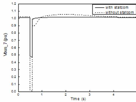
Fig.10: Voltage at bus 7
