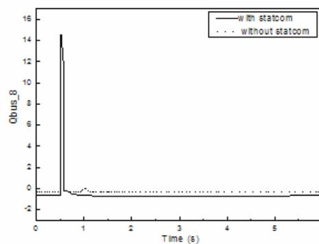
Fig.12: reactive power provided by the statcom at bus 8
