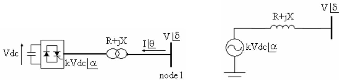
Fig.1 : STATCOM and its equivalent circuit
