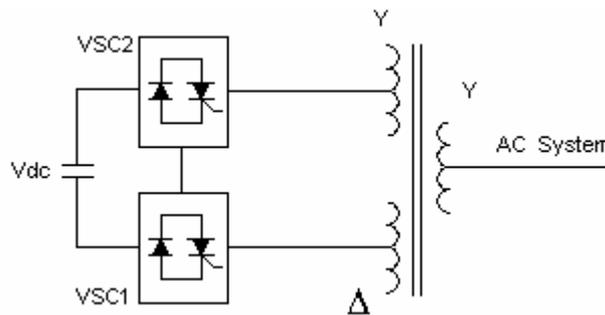
Fig.2 : schema of the 12-pulse STATCOM
